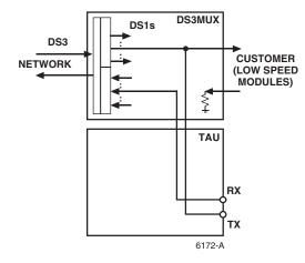
Figure 575-3g. Drop: Network / Insert: Network
